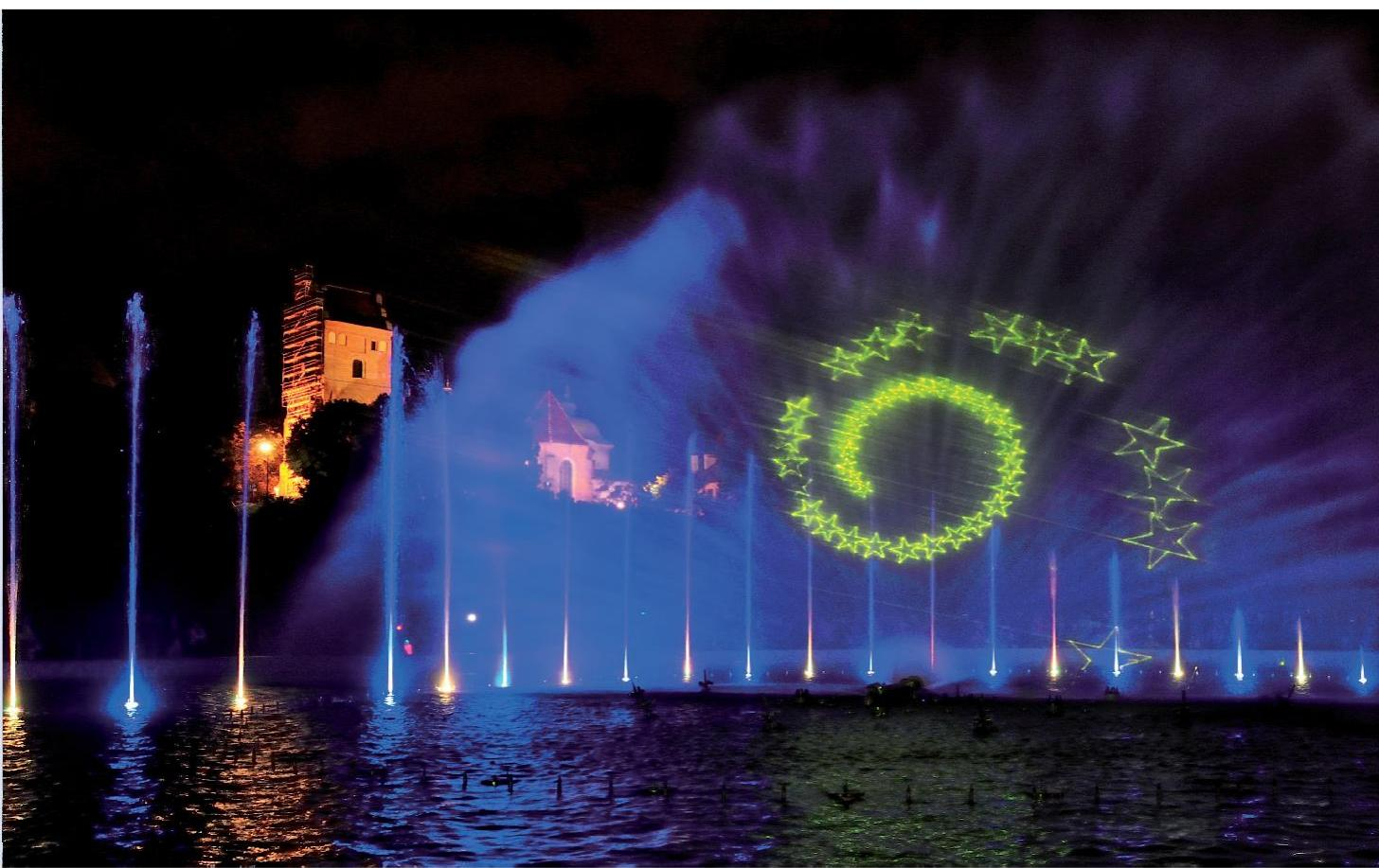
The nozzle creates a filmy WaterScreen. This qualifies for projection of Laser, Video, Slide and Gobo (Graphical optical blackout) type of illumination. Based on the law of physics of light, the position of the nozzle should always be between the viewer and projector.
