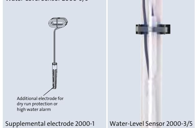
The stainless steel housings of the Water-Level Sensor 20-3 and 20-4 also take on the function of the common electrode. The minimum and maximum electrodes are in the housing. The permanently set level difference is 20 mm. In addition the 20-4 has a dry-run protection electrode.
