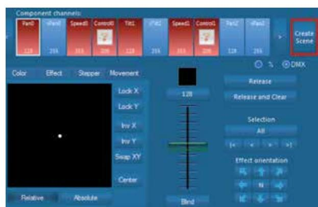
**Effect scenes:** An effect scene consists of a static scene with overlayed and mathematical time function (e.g. sinus, rectangle, saw tooth). Effect scenes changes its value depending on time.
