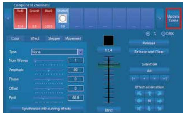
**Dynamic scenes:** A dynamic scene consists of a static scene with a further delay. The delay is splitted equally under selected assemblies and sorted in the order of selection. A static effect which can be used for all selected assemblies is started according to its delays. By this, the gained water picture receives an effective dynamic.
